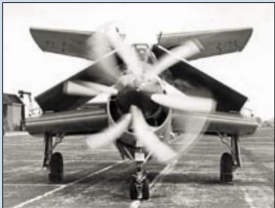
ABOVE With wings fully folded and the contrarotating propellers spinning in opposite directions, the Gannet presented a startling insect-like sight from head-on.
